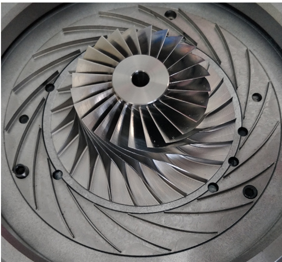
Fig. 1. TTL-1-Scale impeller reversely placed on its casing.
